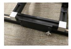
Then pull or push the upper frame into position, grabbing the center vertical beam. Use the tape measure on the right side of the lower frame for precise placement. When the upper frame is in the correct position, tighten both the thumb screws securely. Check that the upper frame is no longer free to slide with a push or pull.
