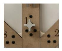
When adjusting the faces, it is crucial that you do not over loosen the thumb screws (pictured to the left). This will cause them to come out of the T-beam at the back of the face. If the thumb screws do come out of the T-beam, align the screw with the hole of the T-beam and screw it back into place.
